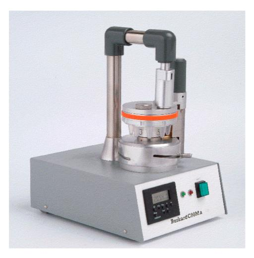
Burkard Indoor Automatic Multi-Vial Cyclone air sampler offers rapid detection of airborne spore and particle matter. Samples are collected into 1.5 Eppendorf vials located on a carousel. Movement of the carousel is by an automatic timer system, or manually through controls on the front panel.
