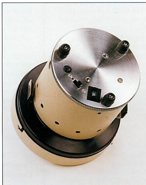
Underside view of air sampler illustrating the timer unit and 'on-off' switch.
