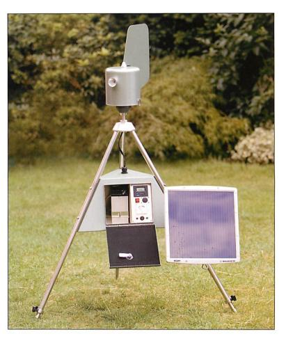
A new 'Multi-vial Cyclone Sampler' for field operation, based on Burkard's miniature cyclone sampler, collects air samples direct into 1.5ml Eppendorf vials. This new facility allows samples to be analysed by a number of techniques including serological (ELISA) and molecular (PCR).
