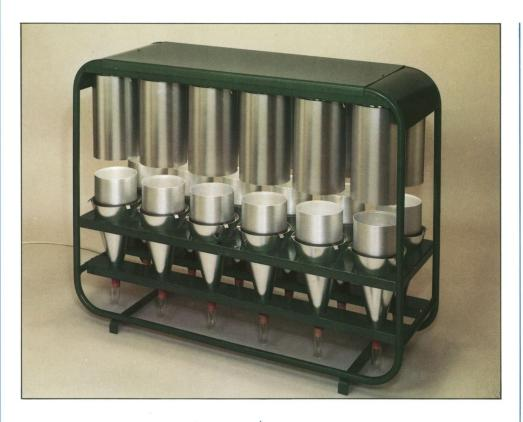
This apparatus is split to facilitate loading and unloading of the sample and a ventilated gap surrounds the sieve preventing condensation below the sample.
